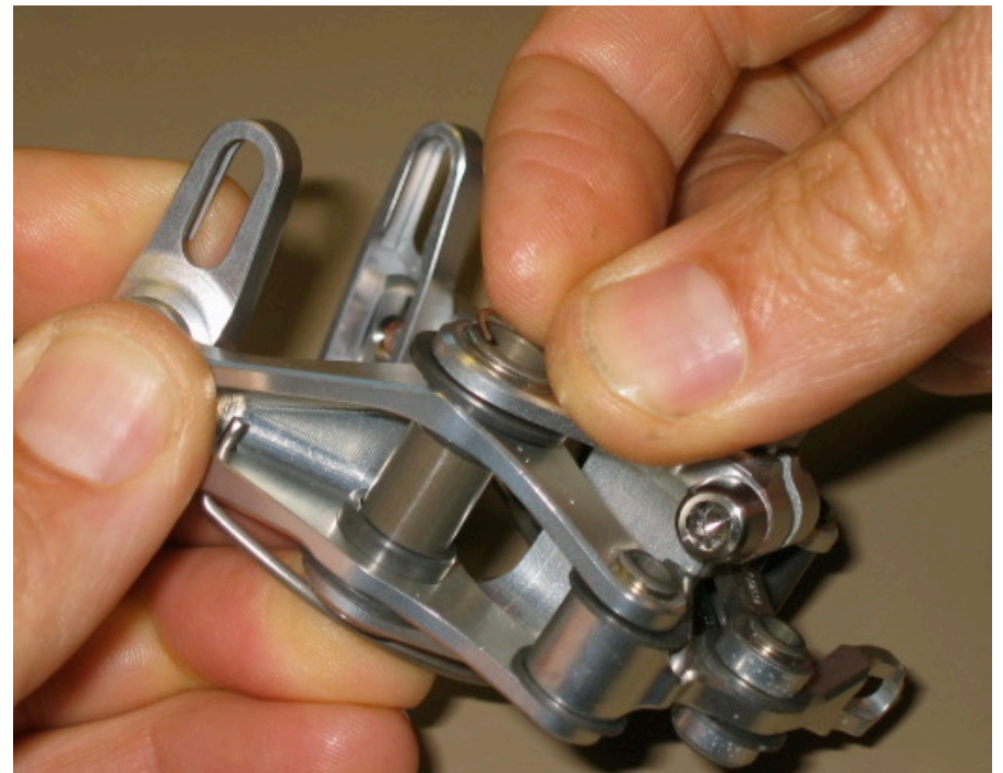
3B. With your fingernail, progressively from the loose end, pull the rest of the ring out of the groove on the axle.
