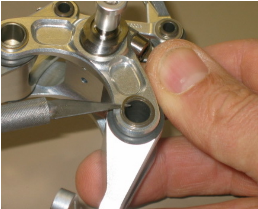
Photo shows end of ring clip out of axle groove.
